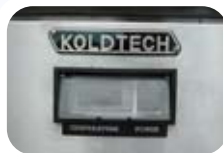
Controller with protective cover to avoid damage from accidental liquid spillage.
